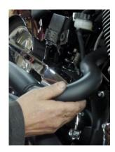
**STEP 6:** Split exhaust clamps are included for both pipes. They are oriented as shown in the inset photo and can be installed on the engine one half at a time. As shown in the main photo this greatly helps the installation of the front pipe. Repeat this process for the rear pipe installation and snug all exhaust flange nuts, but do not tighten them completely.
