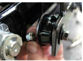
After bracket is installed, slide stock exhaust clamp onto nose of each muffler.
