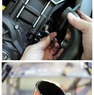
INSTALLING FRONT SHORT HEAD PIPE. Begin by inserting and fitting 02 sensor into 02 sensor port on pipe and tighten into place.
