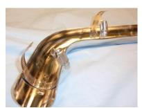
**STEP 5:** The baffles can be installed prior to mounting the pipes to your motorcycle, or once the pipes are in place. Slip the baffles in with the pointed end in first and secure with hardware provided in this kit using an external star lock washers on each screw.
