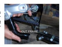
**STEP 3:** Following the procedure outlined in the appropriate service manual for your year and model of motorcycle. Mount frame bracket to rear foot peg hole.
