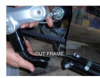
**STEP 3:** Following the procedure outlined in the appropriate service manual for your year and model of motorcycle, remove the swing arm pivot shaft nut. Place the rear mounting bracket over the pivot shaft making sure that the 3/8" washer (inset) is placed inside the bracket as shown, tighten the pivot shaft nut while orienting the mounting bracket facing the rear of the bike, parallel to the ground as shown.
