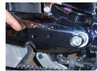
**STEP 9:** Prior to starting the engine, wipe the pipes down with lacquer thinner or acetone on a clean rag. Start your engine and check for exhaust leaks. You are now ready to enjoy your RPW USA Slash exhaust pipes.
