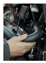
**STEP 7:** Split exhaust clamps are included for both pipes. They are oriented as shown in the inset photo and can be installed on the engine one half at a time. As shown in the main photo this greatly helps the installation of the front pipe. Repeat this process for the rear pipe installation and snug all exhaust flange nuts, but do not tighten them completely.
