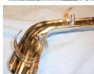
**STEP 5:** The baffles can be installed prior to mounting the pipes to your motorcycle, or once the pipes are in place. Slip the baffles in with the pointed end in first and secure with hardware provided in this kit using two of the external star lock washers on each screw, one on the inside and one on the outside of the pipe.
