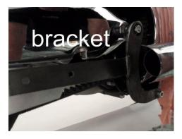
**Step 6.** Next, slip muffler carefully onto header, slowly positioning bracket at same time over mounting studs. Put nuts on pivot shaft making sure that 3/8" washer is on inside of frame bracket. Use large hex head bolts supplied in kit, to frame on bottom of frame bracket. Now you may start tightening all nuts and bolts evenly to secure exhaust pipes to motorcycle.
