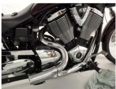
**Step 4.** After head pipes are in place, using the split head clamps as shown, install on the engine one half at a time. Snugly fit all exhaust flange nuts, but do not tighten them completely.
