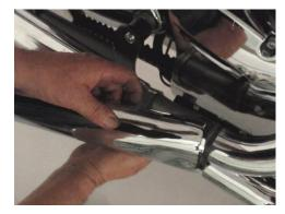
Step 8. Tighten band clamp at muffler to header connection. Tighten head clamps on headers.
