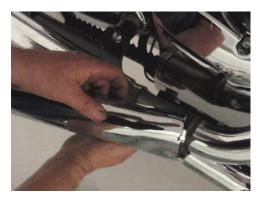
**Step 9**. Tighten band clamp at muffler to header connection. Tighten head clamps on header pipes.
