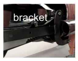
**Step 7.** Next, slip muffler carefully onto header, slowly positioning bracket at same time over mounting studs. Put nuts on pivot shaft making sure that 3/8" washer is on inside of frame bracket. Use large hex head bolts supplied in kit, to frame on bottom of frame bracket. Now you may start tightening all nuts and bolts evenly to secure exhaust pipes to motorcycle.
