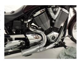
**Step 5.** After head pipes are in place, using the split head clamps as shown, install on the engine one half at a time. Snugly fit all exhaust flange nuts, but do not tighten them completely.
