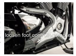
Note: Use blue lock tight on frame bolts to mount frame brackets
