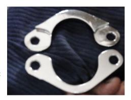
**Step 6:** Undo bolt from frame rail position. Slide mounting bracket up into bolt by sliding on back bolt first. Do not tighten bolts at this time.
