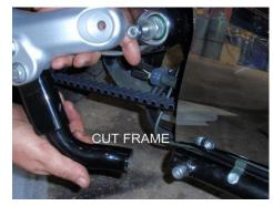
**Step 3.** Installation of the True Dual pipe requires the lower frame rail to be cut off as shown. Save portion that you have cut off. Deburr the frame rail with a file or burr knife to leave a smooth edge and cover any bare metal with touchup paint to prevent rust and plug hole with plastic plug, available at any hardware store
