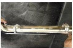
pipe gently away from bike to allow more clearance. Once rear pipe is past fins, finesse rear pipe into rear head port and then maneuver front head pipe into front head port. NOTE: Heat shields must be in place for installation of the primary pipes.
