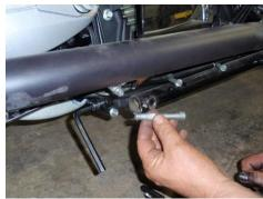
**Step 7.** Put muffler clamp on muffler, slip muffler carefully onto header. Use 5/16"x3/4" bolt to mount muffler to bracket. Now you may start tightening all nuts and bolts evenly to secure exhaust pipes to motorcycle.
