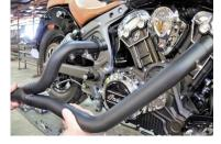
Once rear head pipe is in position, return to front header, snugging up large front head pipe to small front header pipe. Make sure to align T-bolt clamp with end of front header pipe & begin to tighten T-bolt clamp using an 11mm wrench.
