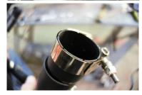
After short header pipe is installed, slip small T-bolt clamp onto front of short section of the large head pipe. Make sure t-bolt clamp nut is positioned on the bottom of the pipe facing out so you can access and tighten later. Align T-bolt clamp with end of pipe & slip large front header pipe with T-bolt clamp onto small header pipe. Do not tighten T-bolt clamp at this time
