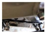
If not using a fuel controller, install 02 sensor reducer plugs to head pipes. Make sure they are screwed in snug.
