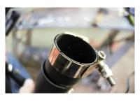
small T-bolt clamp onto pipe. Make sure t-bolt the pipe facing out so bolt clamp with end of
