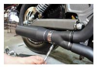
screws with flat and lock washers, tighten bracket to muffler and then tighten your muffler T-bolt clamp onto header pipe making sure edges are aligned with front end of muffler edge.
