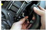
INSTALLING FRONT SHORT HEAD PIPE. Begin by inserting and fitting 02 sensor into 02 sensor port on pipe and tighten into place.
