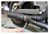
Align bracket with muffler. Slide in muffler bracket insert into back of muffler and attach muffler to mounting bracket using 5/16" x  $^3$ 4 cap screws with flat and lock washers, tighten bracket to muffler and then tighten your muffler T-bolt clamp onto header pipe making sure edges are aligned with front end of muffler edge.
