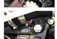
Rotate front and rear exhaust pipes back down seating them into head ports and tighten front and rear head pipe bolts.
