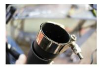
small T-bolt clamp onto pipe. Make sure t-bolt the pipe facing out so bolt clamp with end of
