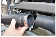
INSTALLING MUFFLER. (Your baffle and endcap have been installed) Slide large T-bolt clamp onto rear muffler. Position T-bolt bolt at bottom of muffler facing out. Slide muffler up onto head pipe as far as you can with muffler bracket at bottom of muffler. You may want to use a rubber mallet to seat muffler all the way onto the collector.
