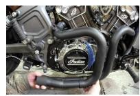
INSTALLING MUFFLER. Your baffle has been installed and you will find that it is loose inside the muffler. (This is normal until installed) Slide large T-bolt clamp onto rear muffler. Position T-bolt bolt at bottom of muffler with screw positioned at the bottom of muffler facing out.
