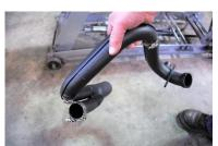
REAR HEAD PIPE. Make sure your heat shield is installed. Put small stainless T bolt clamp onto rear head lower pipe with nut facing down. Carefully slip rear pipe into rear header port area and push forward to seat onto front head pipe. Once seated as far forward as you can go back to rear header port and align rear head clamp with header port. Using OEM nuts secure the rear header pipe to the rear head port and finger tighten nuts
