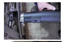
Align muffler mount to bracket on bike. Once aligned attach muffler to mounting bracket using 5/16" x 3/4 cap screw with flat and lock washers, securing muffler to bracket.
