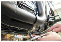
Using an 11mm socket tighten rear header clamp to front header pipe. Secure snugly.
