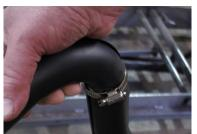
INSTALL BOTH FRONT AND REAR HEAT SHIELDS to front and rear head pipes before fitting pipes onto bike. Make sure the heat shield clamps screw heads are facing down.
