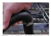
INSTALL BOTH FRONT AND REAR HEAT SHIELDS to front and rear head pipes before fitting pipes onto bike. Make sure the heat shield clamps screw heads are facing down.
