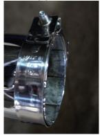
INSTALLING MUFFLER. Your baffle has been installed and you will find that it is secured inside the muffler. Slide large T-bolt clamp onto front section of muffler. Position T-bolt bolt so its positioned with screw positioned at the bottom of muffler facing out.
