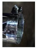
INSTALLING MUFFLER. Your baffle has been installed and you will find that it is secured inside the muffler. Slide large T-bolt clamp onto front section of muffler. Position T-bolt bolt so it's positioned with screw positioned at the bottom of muffler facing out.
