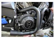
REAR HEAD PIPE. Make sure your heat shield is installed. Put small stainless T bolt clamp onto rear head lower pipe with nut facing down. Carefully slip rear pipe into rear header port area and push forward to seat onto front head pipe. Once seated as far forward as you can go back to rear header port and align rear head clamp with header port. Using OEM nuts secure the rear header pipe to the rear header port and finger tighten nuts
