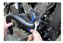
Go back to front header pipe and tighten OEM head nut to factory spec.
