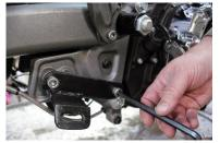
If not using a fuel controller, install 02 sensor "reducer" plugs to head pipes. Make sure they are screwed in snug.
