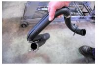
FRONT HEAD PIPE. Carefully slip front head pipe into front head port. Align head clamp with holes and insert OEM nuts. Finger tighten nuts securing front head pipe into place.
