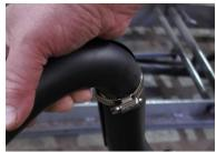
INSTALL BOTH FRONT AND REAR HEAT SHIELDS to front and rear head pipes before fitting pipes onto bike. Make sure the heat shield clamps screw heads are facing down and tail of clamp is tucked under shield before tightening shields to pipes.
