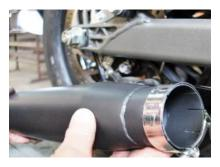
INSTALLING MUFFLER. Your baffle has been installed and you will find that it inside the muffler. Position T-bolt bolt at bottom of muffler with screw positioned at the bottom of muffler facing out.
